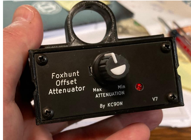
Offset Attenuator (Built ~ $35)
